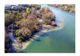
In total, over 15,500 tons of rock, sand and cobble were removed from the channels, 282 small cottonwood and willow trees were planted, and 1.5 acres of land were hydroseeded.
